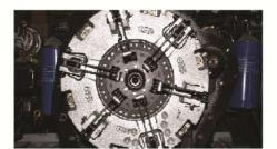
Original import 12 "LUK independent control double acting clutch with large torque reserve coefficient and high reliability
